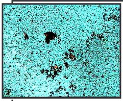
**One mil.** of the sample oil has been forced through a 13-mm diameter **0.3-micron membrane filter** @ 150 P.S.I. The membrane filter has caught any contaminates present, filters are glass slide mounted for examination. This image represents a 1-mm diameter circle focused on the top layer of the filter
