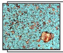
Overview density of dirt, Wear Metal Chunks and debris particles @ 200X.
