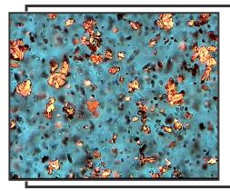
$\label{eq:constraint} \begin{array}{l} \text{Overview density of dirt,} \\ \text{Wear Metal Chunks and debris particles @ 500X.} \end{array}$
