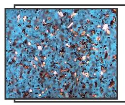
$\begin{tabular}{ll} Overview density of dirt, \\ Wear Metal Chunks and debris particles @ $500X. \end{tabular}$
