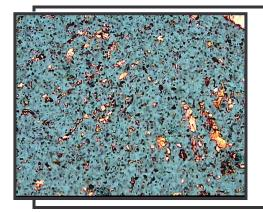
$\begin{tabular}{lll} Overview density of dirt, \\ Wear Metal Chunks and debris particles @ 200X. \\ \end{tabular}$
