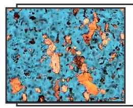
$\begin{tabular}{ll} Overview density of dirt, \\ Wear Metal Chunks and debris particles @ \bf 500X. \\ \end{tabular}$
