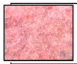
Overview density of dirt, Wear Metal Chunks and debris particles @ 500X.
