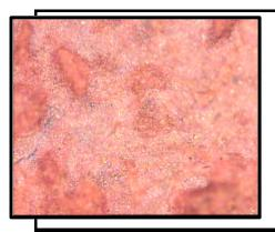
Overview density of dirt, Wear Metal Chunks and debris particles @ **200X.**
