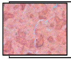
**One mil.** of the sample oil has been forced through a 13-mm diameter **0.3-micron membrane filter** @ 150 P.S.I. The membrane filter has caught any contaminates present, filters are glass slide mounted for examination. This image represents a 1-mm diameter circle focused on the top layer of the filter @ **100X**. The green/blue coloured background is the microscopes bottom light shinning up through the glass slide illus trating density level of dirt, metal chunks and debris particles.
