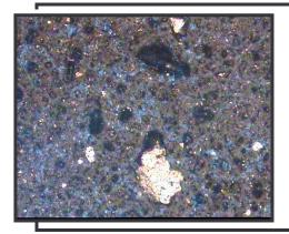
$\hbox{Overview density of dirt,} \\ \hbox{Wear Metal Chunks and debris particles @ $200X.}$
