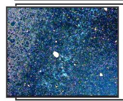
**One mil.** of the sample oil has been forced through a 13-mm diameter **0.3-micron membrane filter** @ 150 P.S.I. The membrane filter has caught any contaminates present, filters are glass slide mounted for examination.
